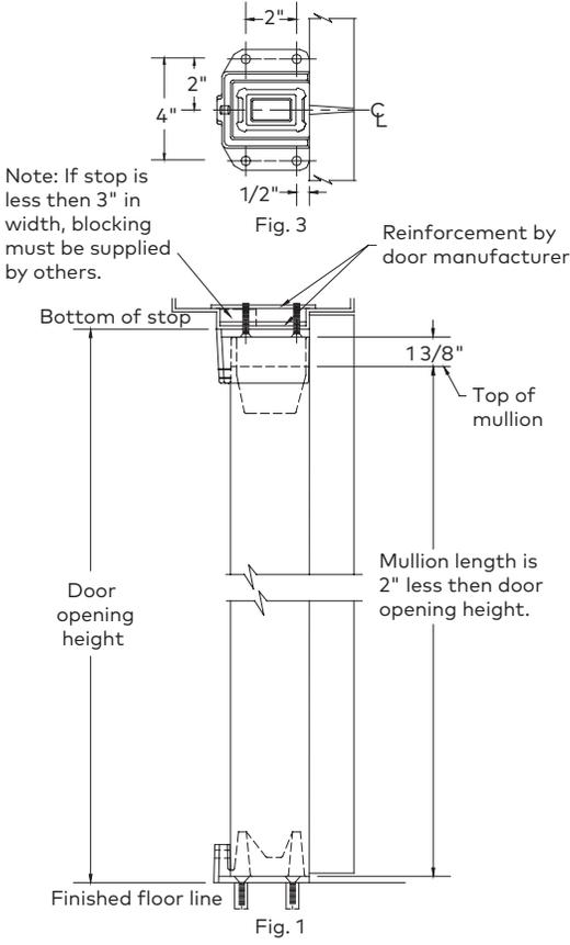
**Step 1:** Measure door opening from finished floor to bottom of stop at centerline of doors. (See Fig. 1) Subtract 2" from this dimension for mullion length. Measure and cut mullion from opposite end marked "Do not cut".
